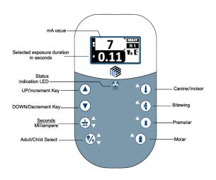
Figure 14. Intraskan DC Keypad Console with LCD Display
