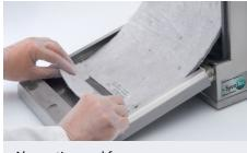
Absorption pad for excess lubricant and debris
